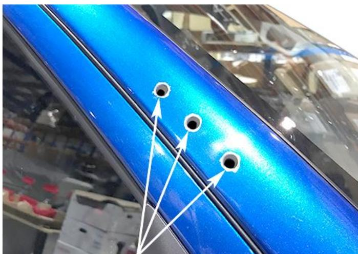
Drill A-Pillar Panel 8mm, Inner Panel 6.5mm
